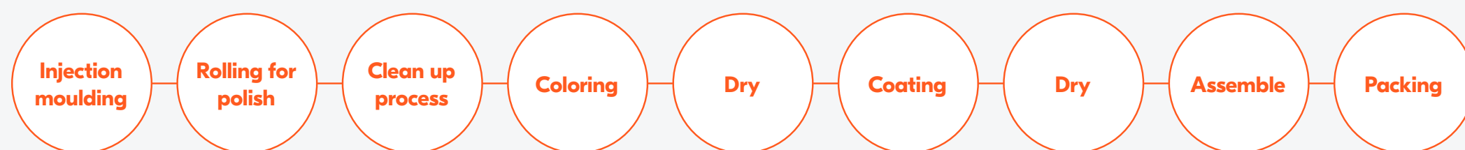
Figure 4 - KASAI eyewear production process flow
